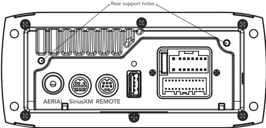
In some cases a rear support strap (not supplied) may be required. Please use the two holes indicated above, to attach the strap using two 8 gauge x 8mm self-tapping screws (not supplied).
