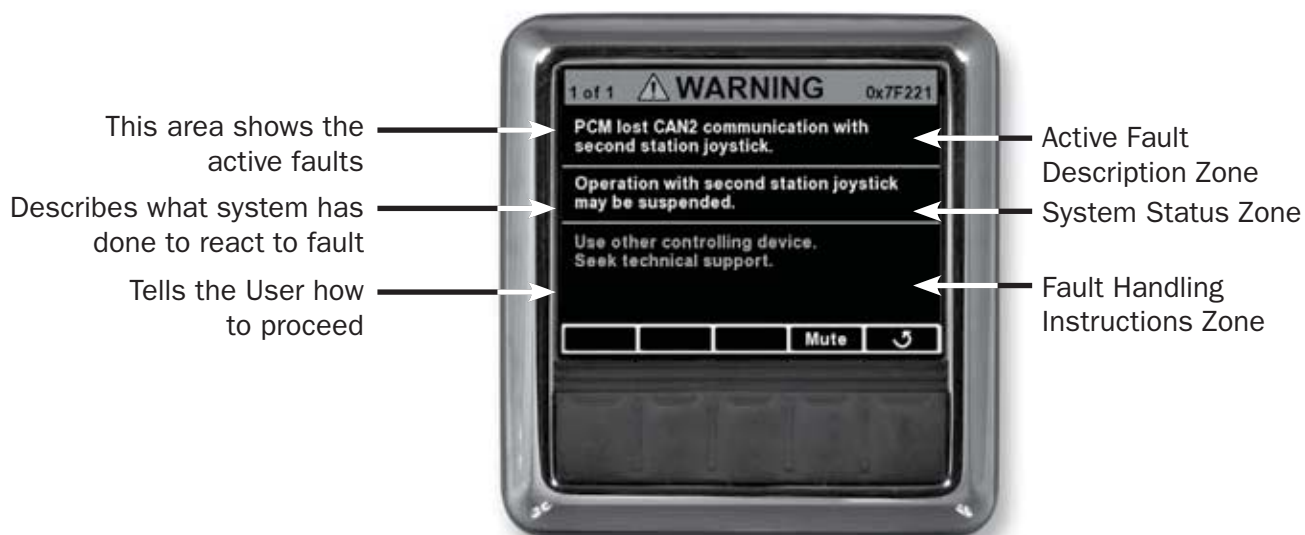
Figure 6-6. Sample warning fault.
