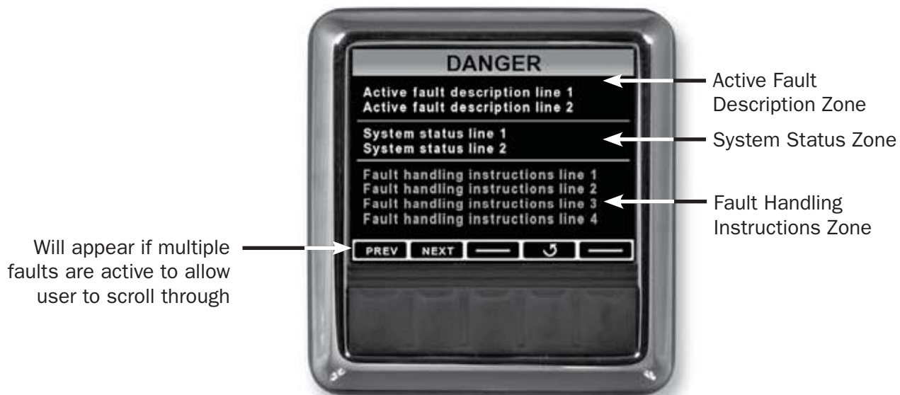
Figure 6-1. Danger fault screen layout.
