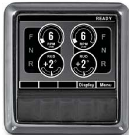
Figure 3-9. All Helms Active screen (normal steering mode).
