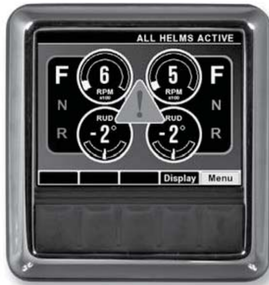
Figure 6-5. Run screen with system warning.
