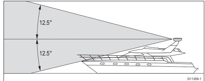
Mount the scanner so that the array rotates parallel to the waterline.
