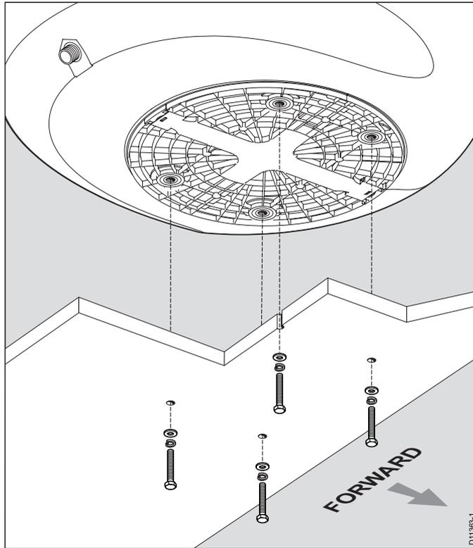
**Note:** The M8 bolts that secure the Digital Radome scanner to the mounting platform require a torque of 20Nm (177lb.in). Use the supplied "Denso Paste" to lightly coat the mounting bolts.
